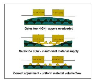
the areas in question. This may be a result of excessive wear or improper adjustment of the paver's material handling components, combined with the inability of a particular mix to flow. The paver must be properly maintained and operated such that an adequate and consistent head of material is delivered to all locations.
