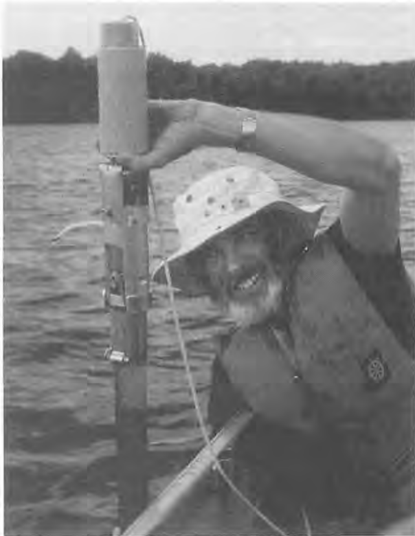
Figure 20-9 A sediment gravity corer with a core visible in the transparent core tube. (Photo courtesy of J. Smol.)
