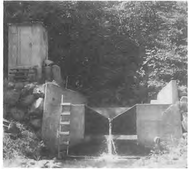
Figure 5-3 A calibrated weir used to determine stream discharge and housing for the water level recorder used to measure changes in discharge over time. (Photo courtesy of J.D. Cunningham, Visuals Unlimited.)
