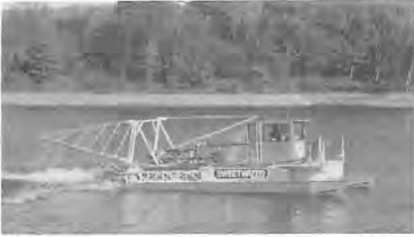
Figure 17-5 Aluminum sulfate (Alum) additions to a eutrophic US lake. The precipitation of phosphorus as \text{AlPO}_4 from the water column and storage in aerobic sediments as \text{AlPO}_4 , \text{FePO}_4 or \text{Fe}(\text{OOH})\text{PO}_4 flocs results in a (temporarily) reduced phytoplankton biomass and increased water transparency. (Photo courtesy of Sweetwater Technology, Division TeeMark Corporation.)
