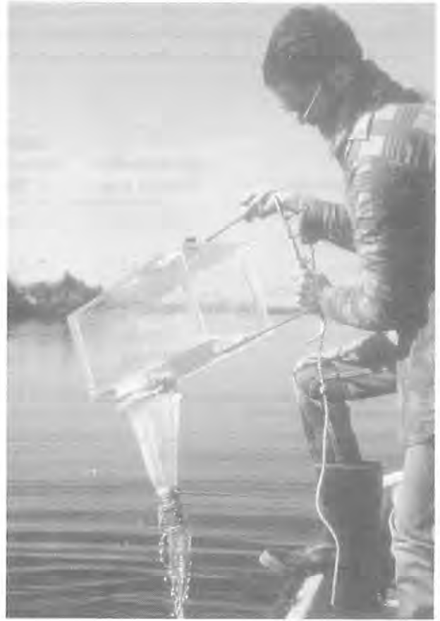
Figure 23–1 A Schindler-Patalas trap for collecting zooplankton. The two hinged doors swing upward when the trap is lowered and close at the desired depth when the hauling-up commences. The organisms contained within the volume (e.g., 30 l) are collected in the attached net. (Photo courtesy of J. Kalff.)
