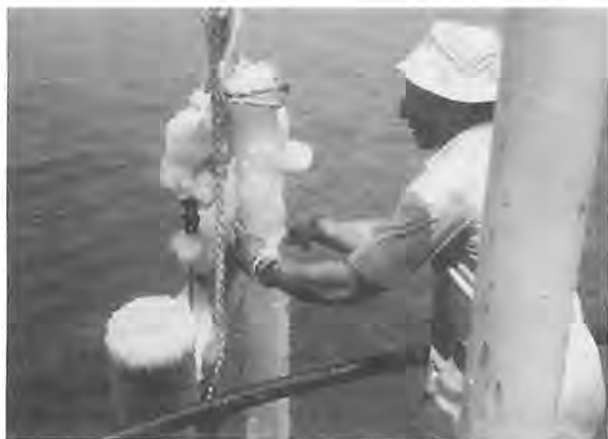
Figure 13-8 A 6 cm diameter thick coating of precipitated salt on an instrument mooring line in the Dead Sea (Israel, Jordan) following a six week exposure. (Photo courtesy of A. Hecht.)
