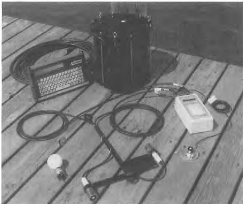
Figure 10-3 Light measuring equipment. In the foreground, a lowering frame holding two cosine ( 2\pi ) underwater quantum sensors to measure the downwelling and the less frequently measured upwelling radiation. Electrical cables connect to a data logger (shown on right) or to a quantum radiometer (not shown) for instantaneous measurements. An above surface quantum sensor is attached to the data logger. To the left of the lowering frame, an almost spherical ( 4\pi ) scalar sensor. At the rear, an underwater spectroradiometer plus a portable terminal. (Photo courtesy of LI-COR, Inc., Environmental Division.)
