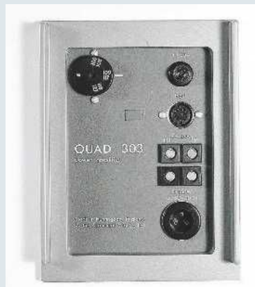
The 'back to front' design means that all sockets are on the front panel
