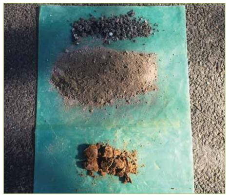
Figure 2.2.9 - BH3: Existing Pavement Materials (Top to Bottom)
