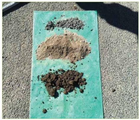
Figure 2.2.6 - BH3: Existing Pavement Materials (Top to Bottom)
