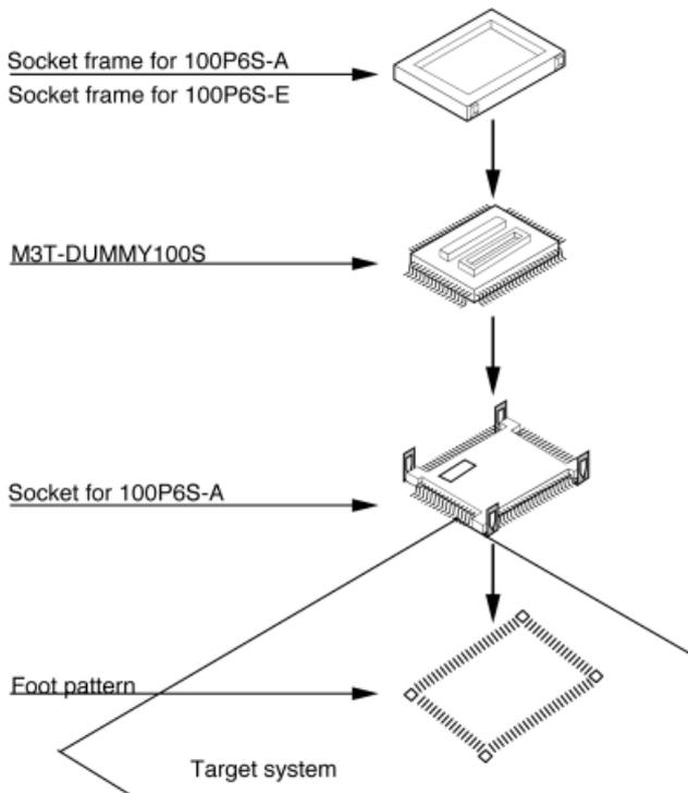
\* The 100P6S-E is an IC package whose lead wire is longer than that of 100P6S-A.
