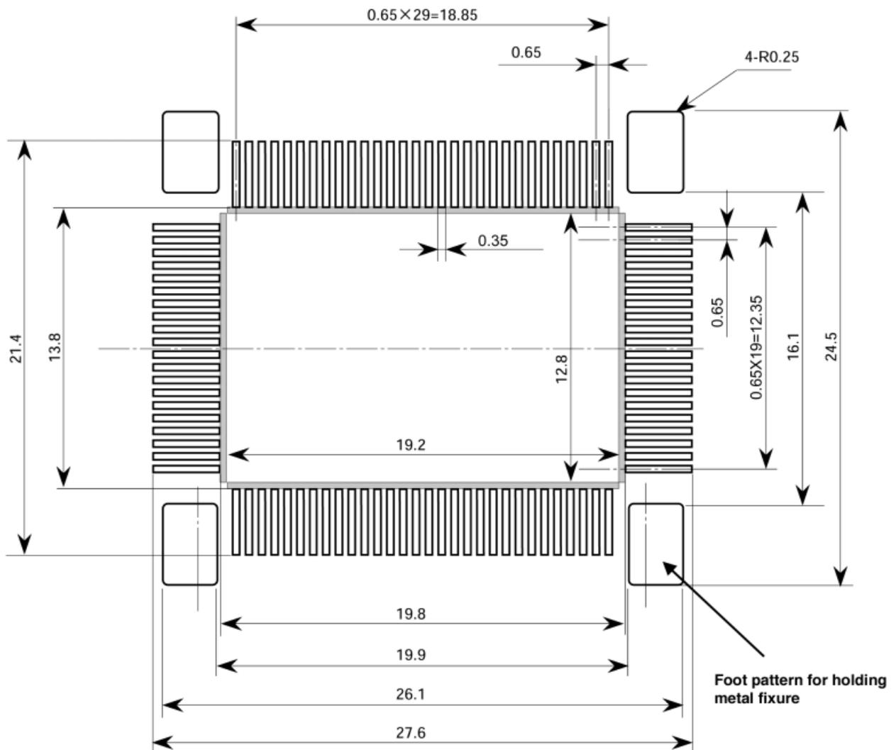
\* When using the AXS4003M295C made by Matsushita Electric Works, Ltd., note that the contacts of the IC socket proper touch the PC board in the shaded section. Therefore, be especially careful with pattern wiring to ensure that other pins will not be shorted. (Through holes are not accepted.)
