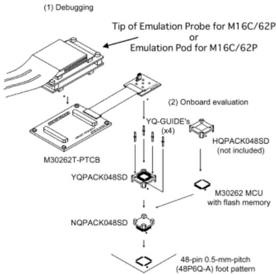
\*: No. 1 pin position Be sure to align the pins.
