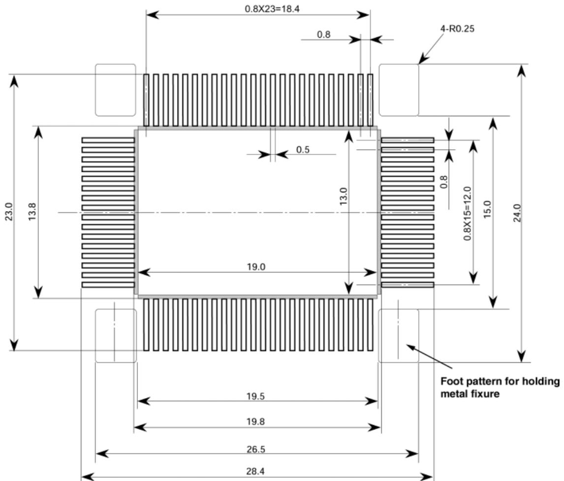
\* When using the AXS4803M19 made by Matsushita Electric Works, Ltd., note that the contacts of the IC socket proper touch the PC board in the shaded section. Therefore, be especially careful with pattern wiring to ensure that other pins will not be shorted. (Through holes are not accepted.)
