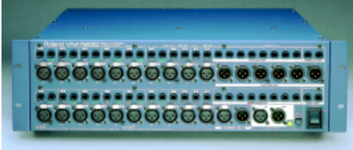
All of the actual mixing takes place within the V-Processors: The 48-Channel VM-7200 (above) or the 24-Channel VM-7100, where you'll find all the ins and outs you need
