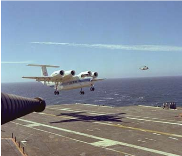
The NASA-Ames Quiet Short-Haul Airplane lands on the carrier Kitty Hawk without arresting gear in 1980.
