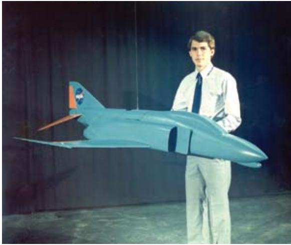
Langley researcher David E. Hahne poses with F-4 free-flight model, shown in flight at high angles of attack in the Langley Full-Scale Tunnel.
