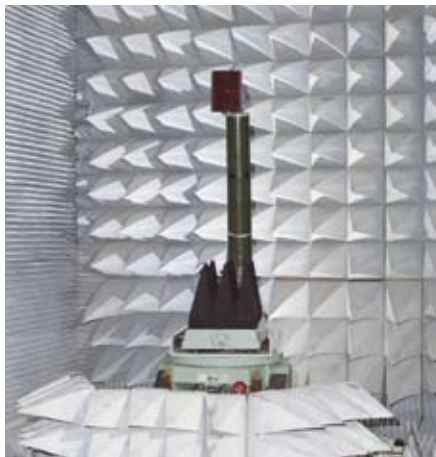
Brassboard testing of Joined-Wing Flight Demonstrator array element at Langley
