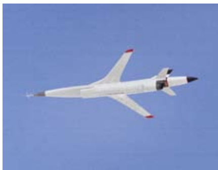
Drone during flight with ARW-1 research wing on June 12, 1980, before catastrophic flutter occurred.
