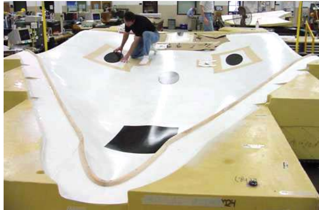
Construction of the Blended Wing Body Low-Speed Vehicle in a Langley shop.
