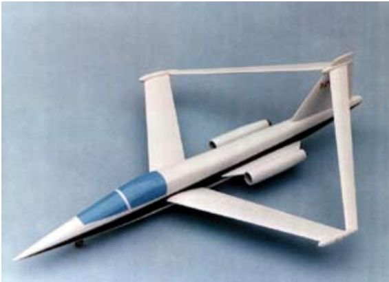
Model of the Ames Joined-Wing Research Aircraft concept shows two of the three wing arrangements.
