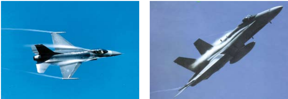
The F-16 (left) and the F/A-18 (right) use vortex lift for improved maneuverability.
