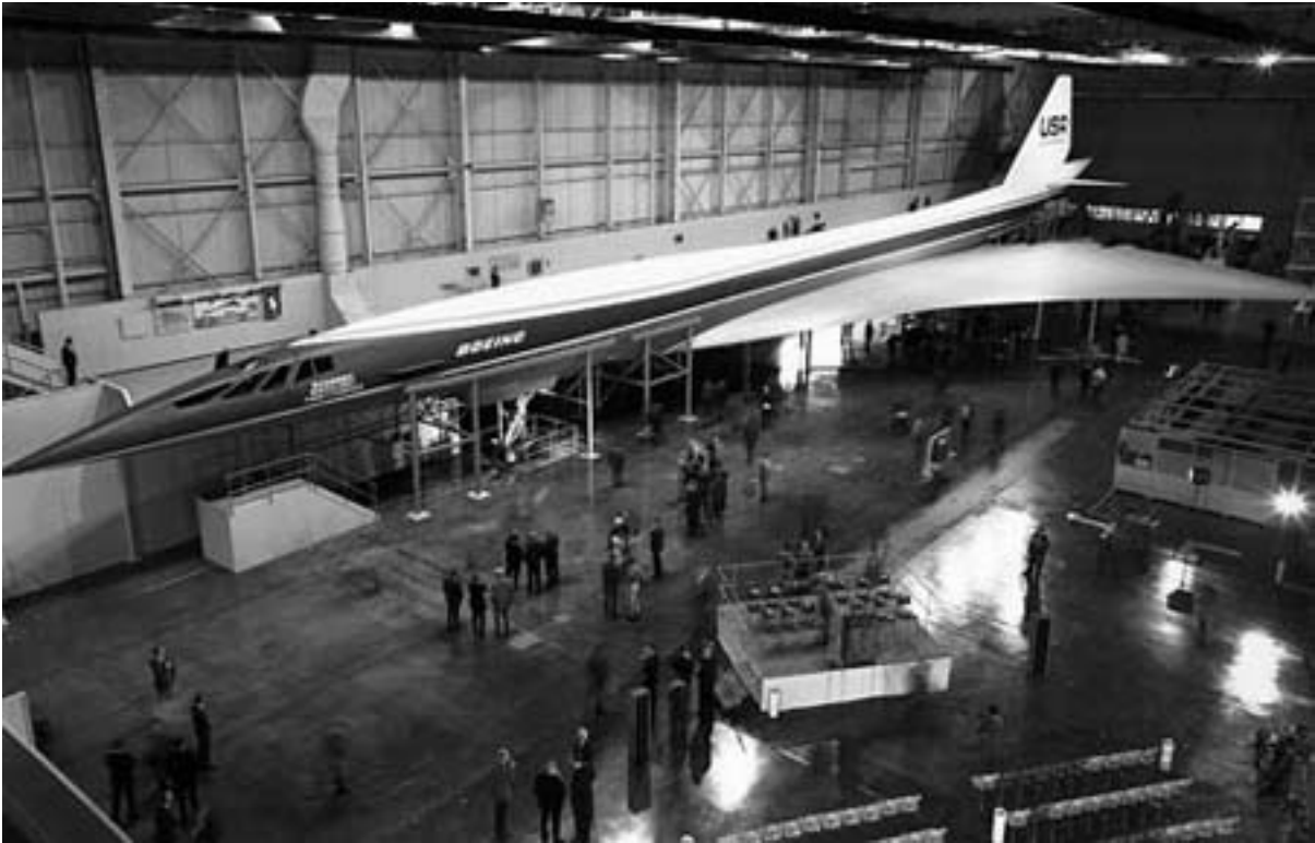
Engineering mock-up of the Boeing 2707-300 Supersonic Transport.
