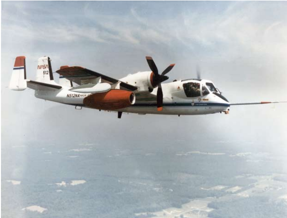
The NASA OV-1B in flight with an NLF nacelle under the right wing. Note feathered propeller and underwing pod containing noise source.
