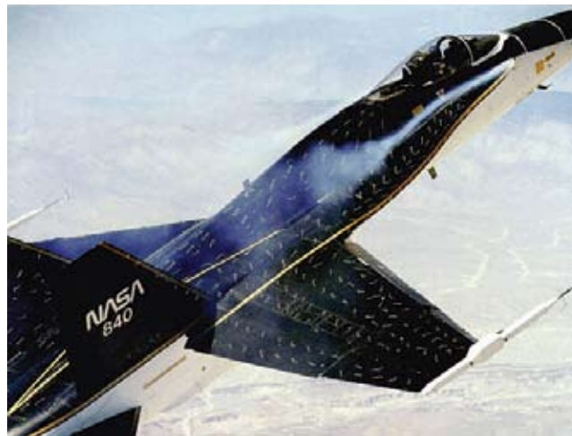
NASA's F/A-18 High Angle of Attack Research Vehicle uses smoke injected into vortex flow to illustrate vortex breakdown position for angles of attack of 20 degrees (top) and 30 degrees (bottom).
