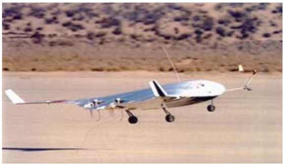
The 6-percent remotely controlled blended wing body model flown by the Stanford University Advanced Concepts for Aeronautics Program team.
