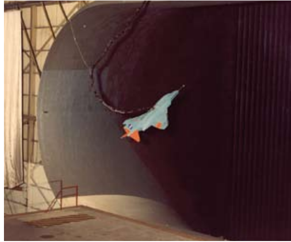
Langley researcher David E. Hahne poses with F-4 free-flight model, shown in flight at high angles of attack in the Langley Full-Scale Tunnel.
