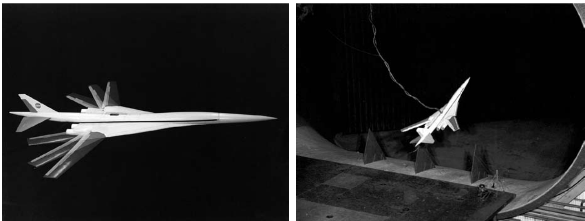
Time-lapse photography shows the variable sweep wing of early Boeing Model 733-290 Supersonic Transport design. Free-flight testing was conducted in the Langley Full-Scale Tunnel.
