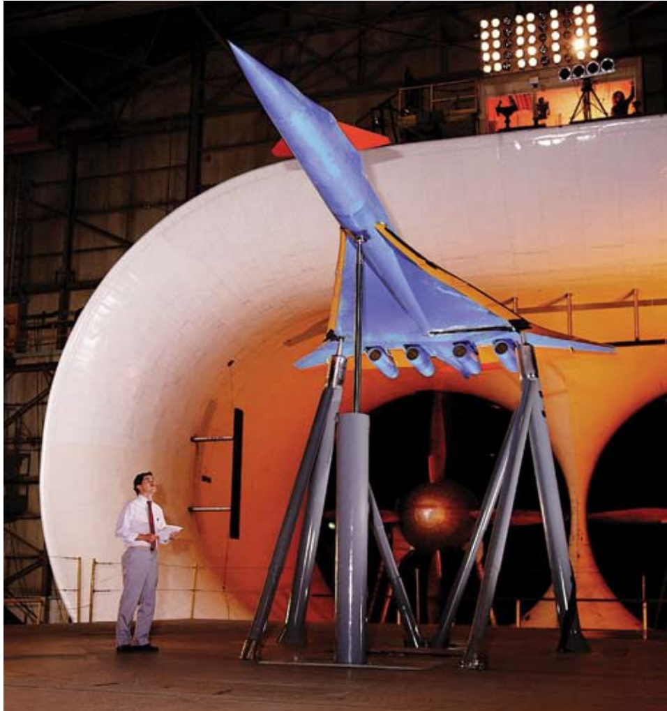
Researcher David E. Habne inspects a 1/10-scale model of a McDonnell Douglas Mach 2.2 transport in the Full-Scale Tunnel in 1992.
