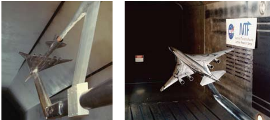
Extensive testing of the High Speed Research Reference H configuration was conducted in many Langley tunnels, including the 16-Foot Transonic Tunnel (left) and the National Transonic Facility (right).
