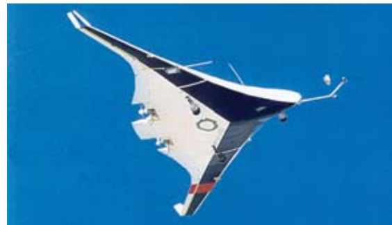
The 6-percent remotely controlled blended wing body model flown by the Stanford University Advanced Concepts for Aeronautics Program team.
