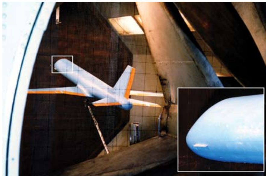
Model configuration tested in Strake Technology Research Application to Transport Aircraft project.
