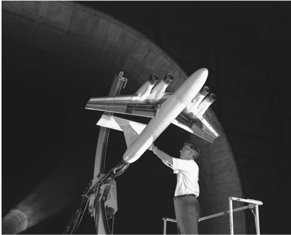
Full-span four-engine upper-surface blown model in the Langley Full-Scale Tunnel.
