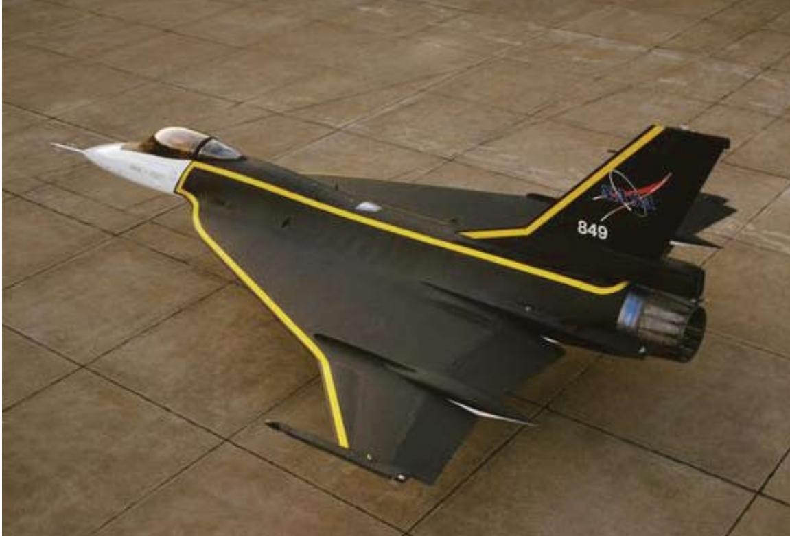
F-16XL aircraft painted by Langley for flow visualization tests.
