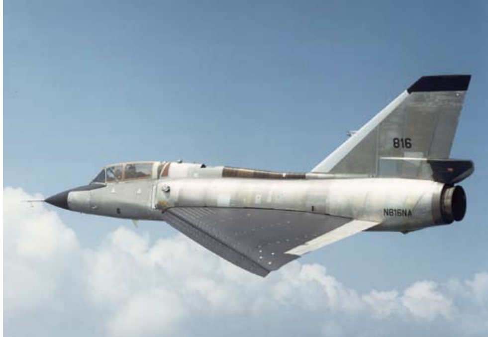
The NASA F-106B in flight with the vortex-flap modification.
