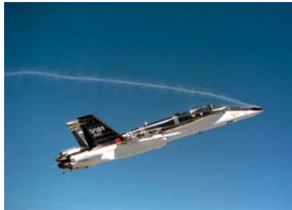
In-flight pictures of the High Angle-of-Attack Research Vehicle showing the right strake deployed (left) and smoke-flow visualization of the vortex path shed by the strake (right)
