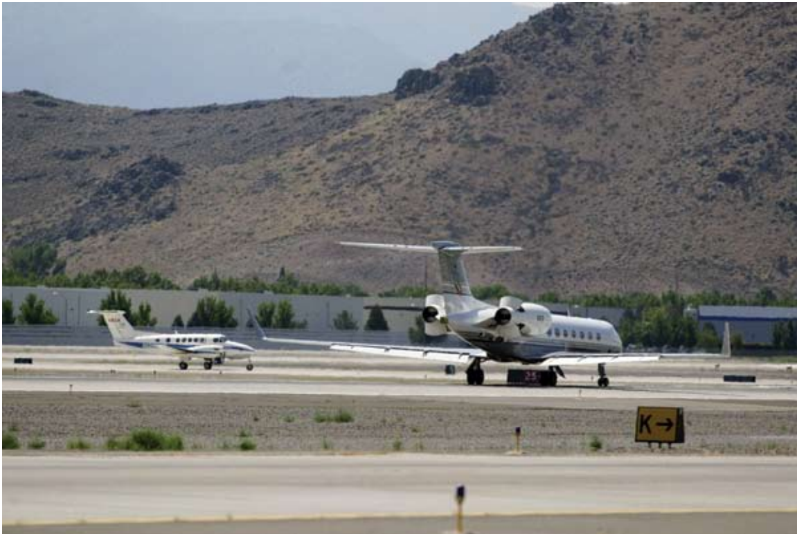
Simulated runway incursion by NASA King Air airplane (left) during Reno evaluations of incursion prevention systems on Gulfstream V airplane (right). Note the deployed engine thrust reverser doors on the Gulfstream V as the pilot takes corrective actions to avoid the potential collision.
