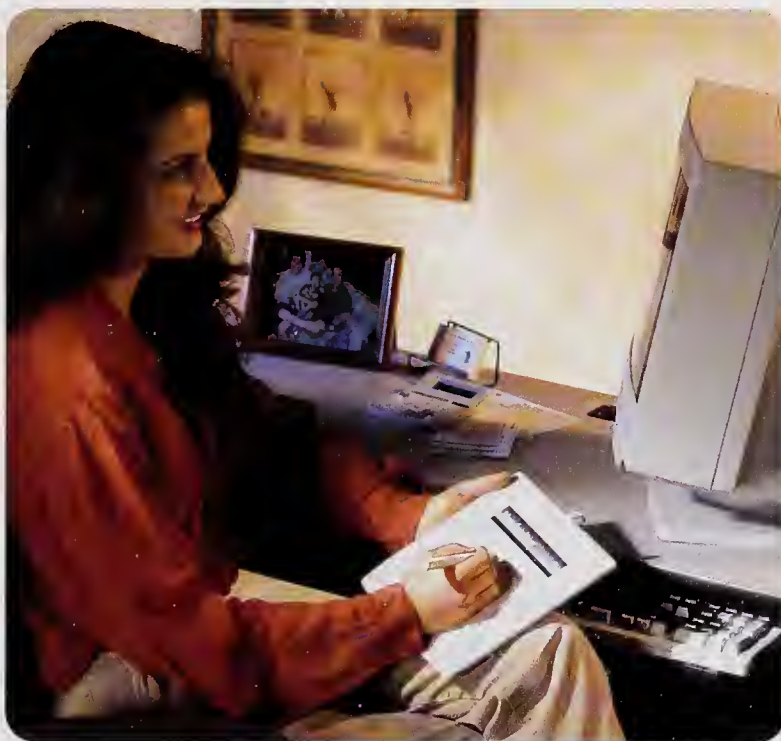
A computer user entering information into her PC with a pad and stylus. Company software in the PC converts the data from the pad into letters and words.
