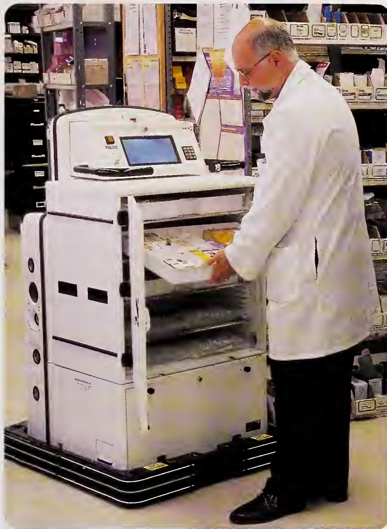
Drugs are loaded on the HelpMate robot by a hospital pharmacist for delivery to staff in one of the hospital's wards.
