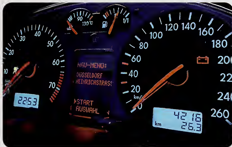
Cree's LED chips are used by Siemens A.G. for back lighting for this dashboard.
