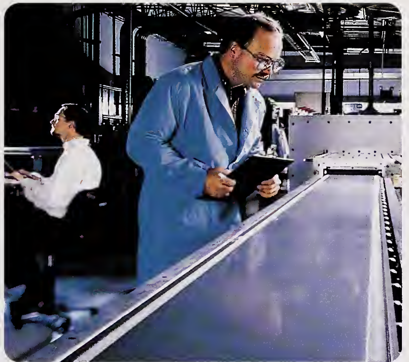
A large area solar grade silicon sheet emerging from a silicon growth reactor which incorporates new ATP-funded technology.
