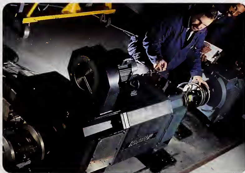
A 286 hp demonstration motor constructed by Reliance Electric with HTS windings supplied by ASC.
