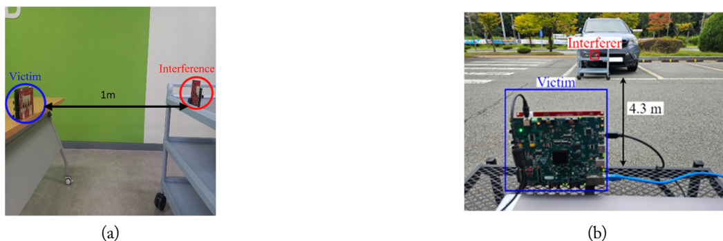
Fig. 5. (a) Interferer (AWR2944) and victim (AWR2243) radars and the indoor laboratory experiment's environment. (b) Outdoor environment with increased distance and a stationary vehicle.
