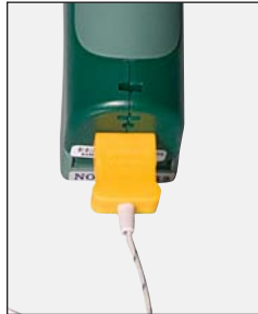
Type K input for contact measurements
