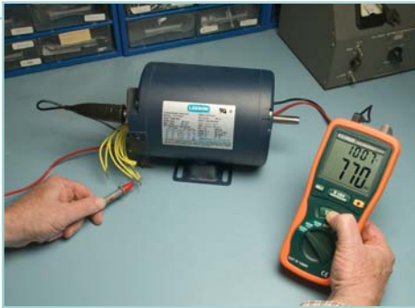
Measures the insulation resistance of motors.
