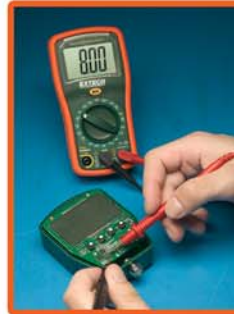
Autoranging Automatically selects the optimum measurement range for accurate readings
