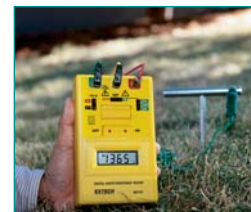
Check resistance between earth and grounding rod.
