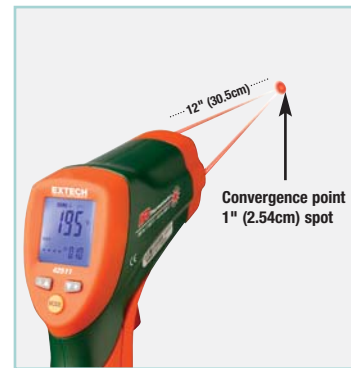
42511 12" Distance IR Meter When measuring at 12" (30.5cm) distance, laser convergence pinpoints your exact target spot of 1" (2.54cm)
