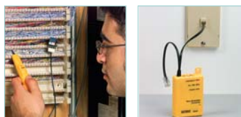
Transmitter injects traceable signal into cables, checks telephone lines, and performs continuity checks
