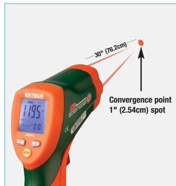
42512 30" Distance IR Meter When measuring at 30" (76.2cm) distance, laser convergence pinpoints your exact target spot of 1" (2.54cm)
