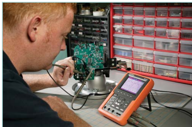
Dual trace testing or troubleshooting of printed circuit boards and electronic assemblies
