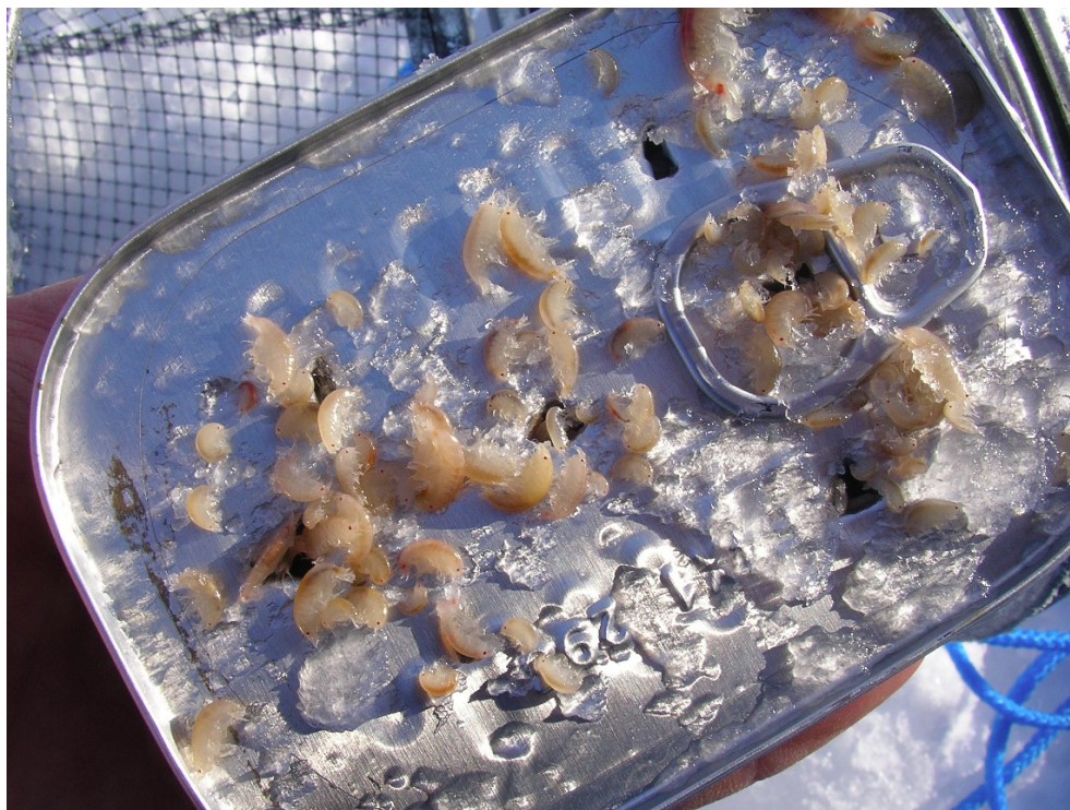
Figure 6. Sardine cans with the lids pictured were used as bait in Gee minnow traps deployed under the Beaufort Sea ice. This method allowed the scent of the bait to escape and inadvertently acted as an amphipod trap within the minnow trap.
