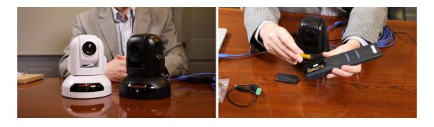
**Step 5:** Let's test out the camera's PTZ functionality with the included IR remote control. Start by inserting the included AAA batteries into your IR remote control. Now you can operate the Pan, Tilt and Zoom of your camera using the IR Remote. Let's set a camera preset to familiarize ourselves with the remote control. First click the number you would like to save a PTZ preset for
