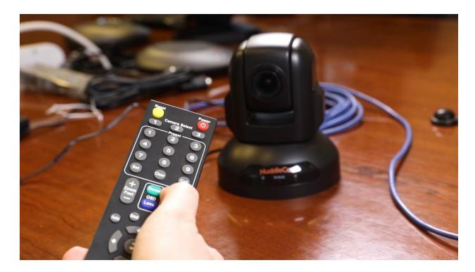
**TIP:** If your remote control is not controlling your camera, double check the IR address your camera is set to. The default address is 1. Let's press the number 1 button on the top of the IR remote control to make sure the IR remote is set correctly.
