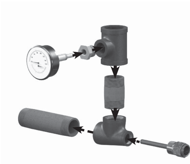
Figure 3 - Temperature Pressure Gauge
