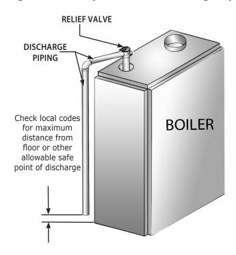
Figure 3 - Forced Hot Water Typical Piping
