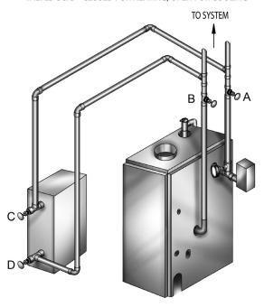
Figure 6 - Bypass Piping
