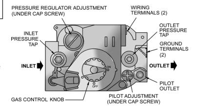
Figure 13 - Pilot Flame Adjustment
