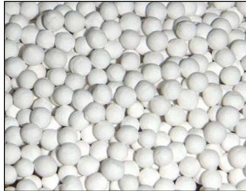
Figure 13. Alumina balls, a high-temperature candidate sensible thermal energy storage material
