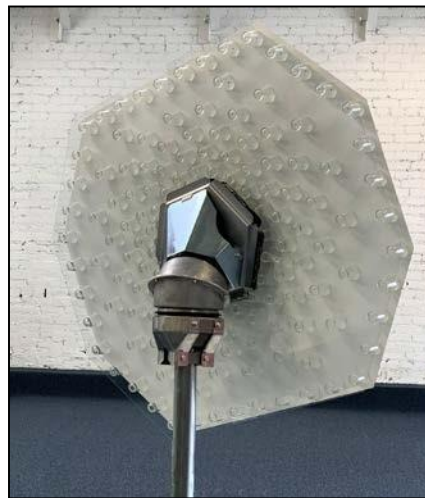
Figure 8- Edison's ~2 m 2 heliostat design, incorporating multiple design innovations that simultaneously improve reliability and reduce cost. The faceted outline serves to eliminate reflector area in the regions of greatest shading and blocking in the optimally-packed heliostat field, thereby further reducing the overall cost-per-kW-delivered
