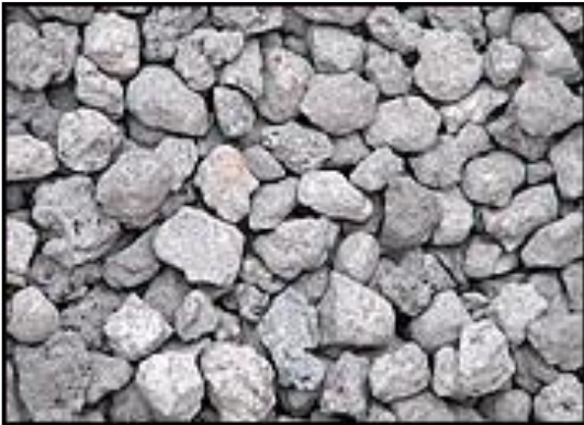
Figure 12. Steel slag, a low-cost candidate sensible thermal energy storage material
