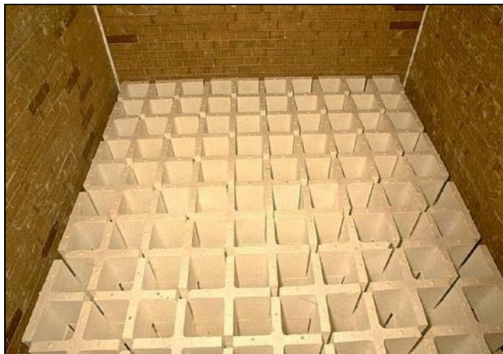
Figure 11. A stacked arrangement of cruciform-shaped firebrick of the type described in [10]
