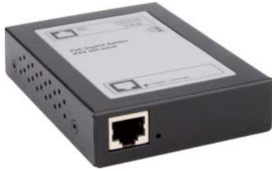
PS-201C 1-port Gigabit IEEE 802.3at PoE+ Injector
