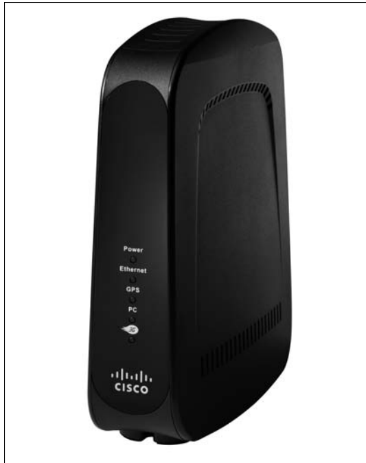
Figure 13-2: Femtocells plug into your home wireless router and give you your own cell tower!
