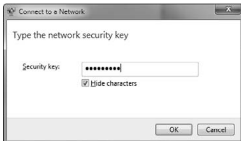
Figure 7-7: Enter your security key (WPA or WEP pass- phrase) in this box.
