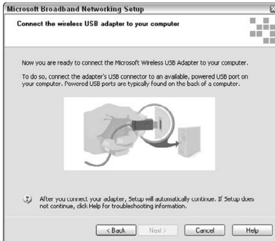
Figure 7-1: Don't connect your wireless network adapter until you're prompted by the setup software.
