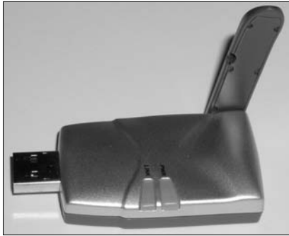
Figure 3-3: Use a USB adapter to add Bluetooth capability to a desktop or laptop PC.
