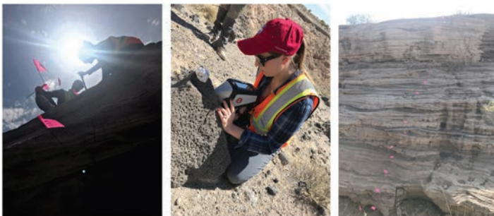
Figure 2: April 2018 field campaign. Left: Transect planning through layered ash deposits. Center: Project ESPRESSO postdoc Marcella Yant performs LIBS measurement of a basalt boulder near Kilbourne Hole. Right: Layered ash transect with LIBS and XRF sample sites marked; vertical extent approximately 6.5 meters.
