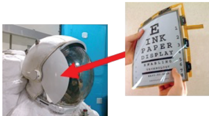
Figure 7. Extravehicular Mobility Unit manually-deployed pull-down sunshade where electrochromic polymer displays will be used.
