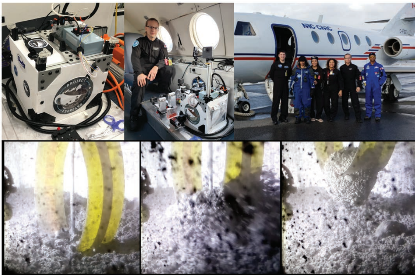
Figure 1: October 2018 reduced gravity flight campaign. Top left and center: Airborne Space Environment Chamber demonstration experiment, mounted to the floor of the NRC-CNRC Falcon 20 reduced gravity research aircraft. Top right: A contingent of Project PoSSUM flight crew and Project ESPRESSO PI Parker. Bottom panels: Sequence of sample extraction of CI Chondrite simulant material using a magnetic grapple under vacuum and microgravity conditions.
