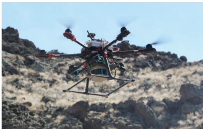
Figure 1.4. Astrobotic field-tested their autonomous navigation capabilities at Aden Crater, NM. The geologic features in the region (lava pits and tubes) are analogs for GPS-denied environments on the Moon and Mars.
