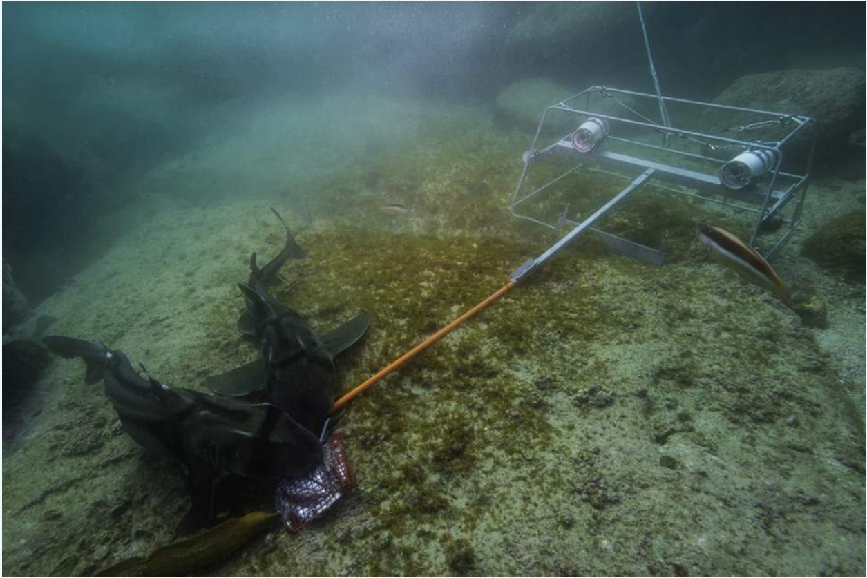
Above. A baited remote underwater video on the seafloor on a NSW coastal reef. These baited systems attract fishes into the bait so they can be identified, counted and measured to assess the condition of the fish assemblages on rocky reefs along the NSW coastline. This image shows two Port Jackson sharks and a green moray eel at the bait bag while a maori wrasse swims past the stereo-video camera system.
