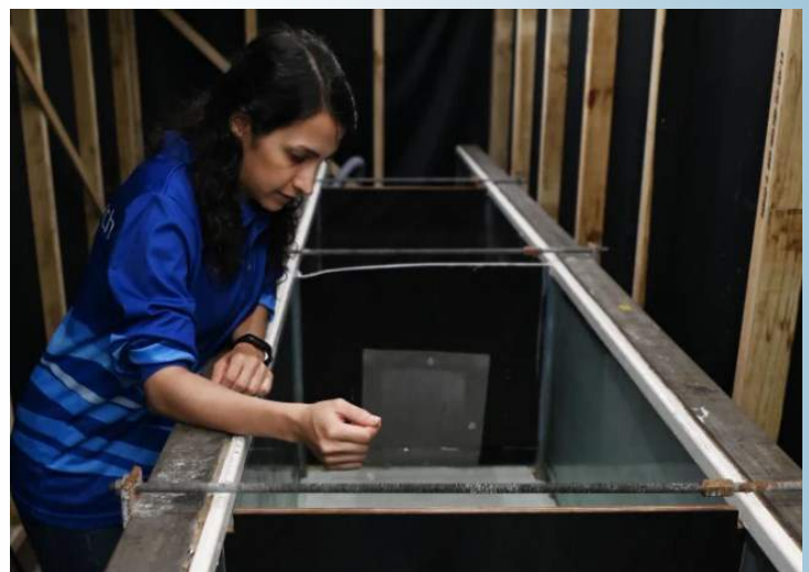
Above. Maryam conducting laboratory experiments to attract freshwater fish species into the UNSW Tube Fishway. Photo taken by Nick Moir
