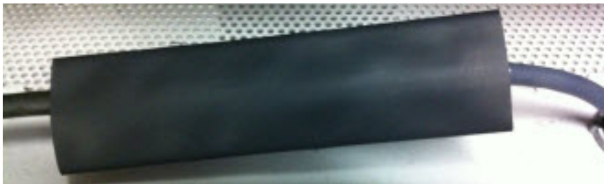
Figure 3-2. Relay and DC Output Cable in Shrink Wrap
