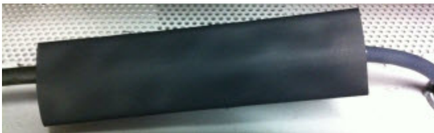
Figure 4-2. Relay and DC Output Cable in Shrink Wrap
