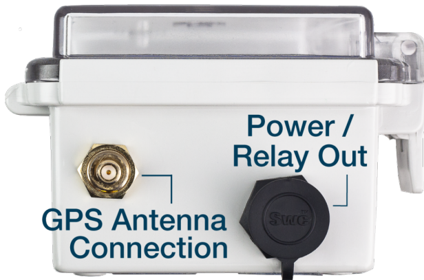
Figure 2-1. GPS Antenna Connection
