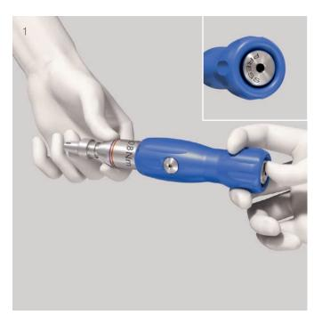
The torque limiter prevents over-tightening and the VA locking screws are securely locked into the plate. (2)
