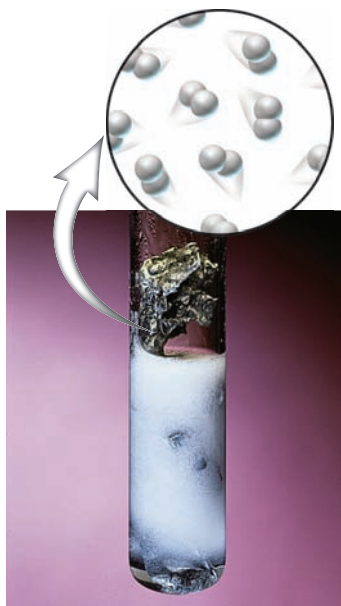
▲ Reaction of Zn Metal Zinc metal reacts with hydrochloric acid to give ZnCl and H 2 bubbles.
