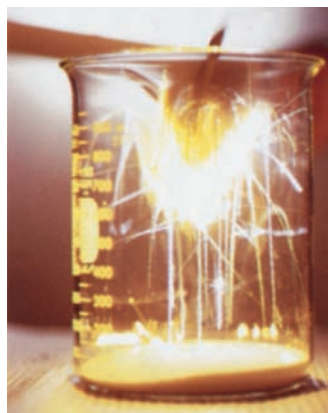
◀ Iron in Oxygen Gas Iron wool reacts in oxygen gas to give bright white light and a gray \text{Fe}_2\text{O}_3 residue.
