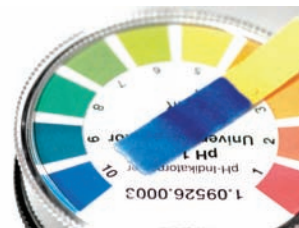
▲ pH Test Strip The indicator test strip paper uses universal indicator to test for pH. The test strip shown indicates a base at pH 10.
