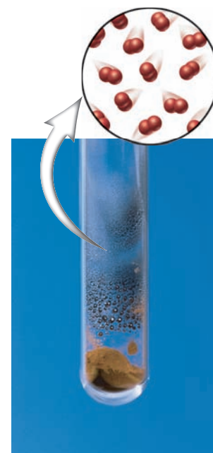
▲ Decomposition of HgO Orange mercury(II) oxide decomposes by heating to give droplets of silver Hg liquid and O 2 gas.
