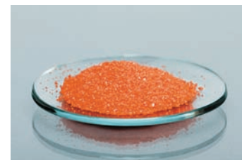
▲ Potassium Dichromate Orange crystals of potassium dichromate dissolve in water to give, K_2Cr_2O_7(aq) .
