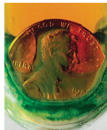
▲ Figure 17.3 A Penny in Nitric Acid The copper penny reacts with nitric acid, \text{HNO}_3 , to give a green solution and brown \text{NO}_2 gas.
