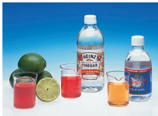
▲ Common Acids Methyl red indicator is added to beakers of lime juice, vinegar, and club soda. The color of the indicator shows a different pH in each beaker.
