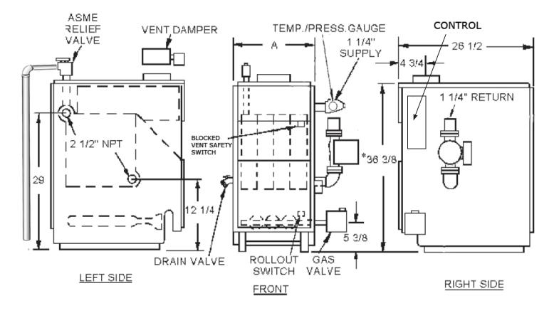
\* Minimum acceptable height for low water cutoff probe.
