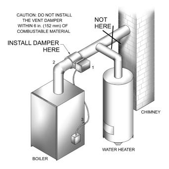
Annually check vent damper and all flue product carrying areas of appliance, with particular attention given to deterioration from corrosion or other sources. If you see corrosion or other deterioration, contact your heating contractor for repairs. Check vent damper operation as follows:
