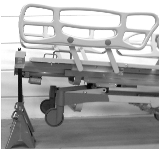
JACK STANDS POSITIONED UNDER THE FOOT END OF THE BED
