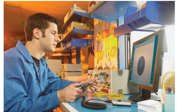
Patchcord inspection in a manufacturing environment
