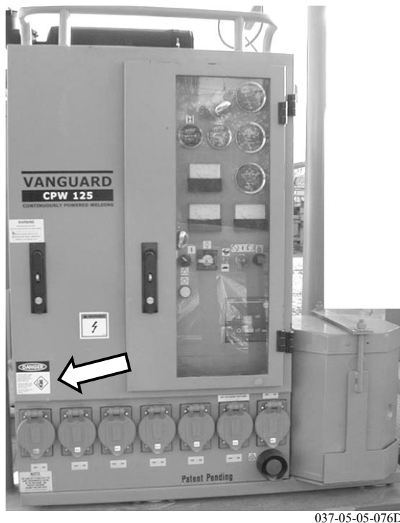
Figure 1: Danger, hazardous voltage, qualified personnel only; located on main door—control/distribution center.
