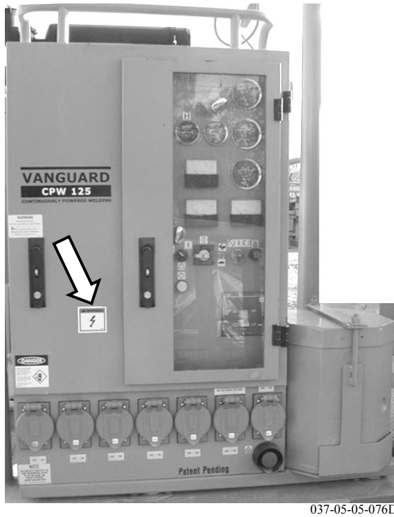
Figure 2: Warning, high voltage electrocution hazard; located on main door control/distribution center, and on rear of control/distribution center.
