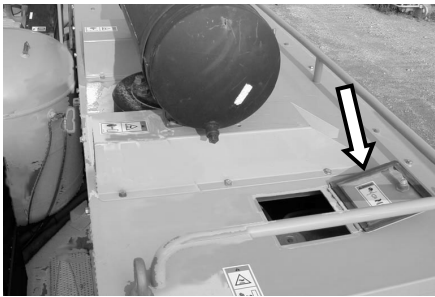
Figure 9: Warning, pressurized coolant, hot surface, read the manual; located on underside of radiator fill door—genset
