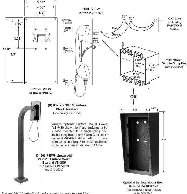
\* **Note:** The gel-filled (water-tight) butt connectors are designed for insulating displacement on 19-26 gauge wire with a maximum insulation of 0.082 inches. Cut off stripped wire ends before terminating.
