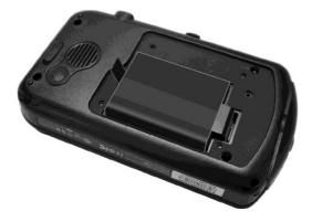
3. Replace the battery cover and tighten the four screws.
