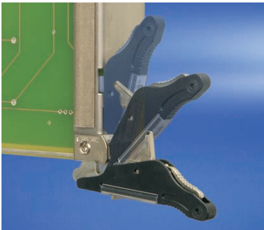
AdvancedTCA spring-loaded IEA handle
