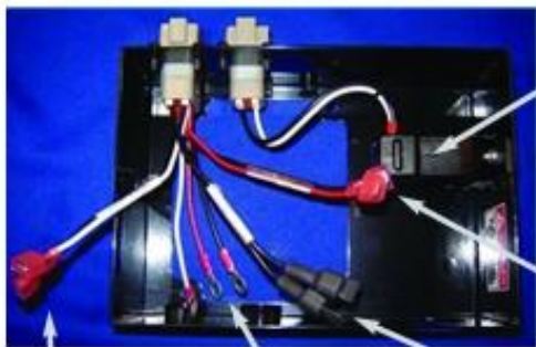
View of Terminal Box
