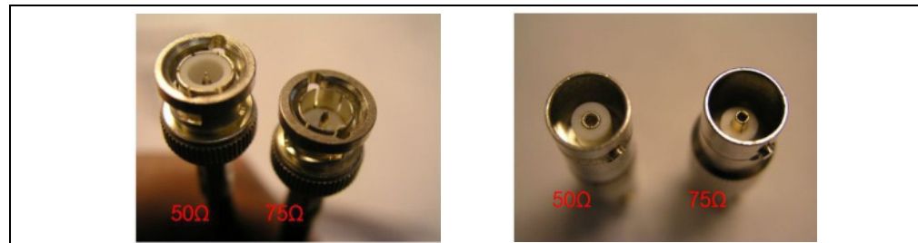
FIGURE 1-3: 50Ω COAX VS 75Ω COAX
