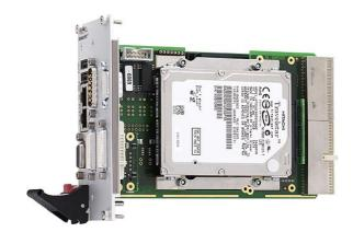
The F601 is a multimedia extension card for 3U Intel® based CompactPCI® single-board computers. It can be used in combination with the F14 and compatible CPU boards.
