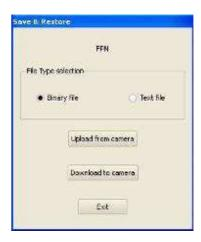
This will allow the user to upload/download out/in the Camera the FFC coefficients in/from a binary or text file that can be processed externally.
