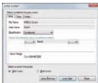
[ Value search ] Values are searched, and the cursor jumps to the position where the conditions match.
