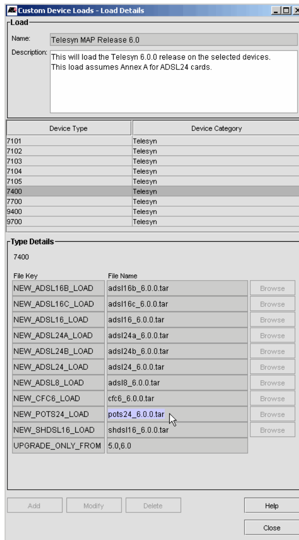
FIGURE 9-56 Details Display for Standard Load (Used to Create Custom Load of Only Certain Files)
