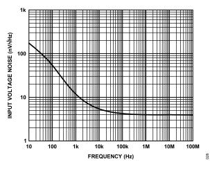
Figure 28. Input Voltage Noise vs. Frequency
