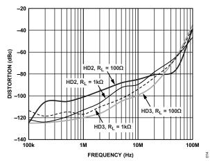
Figure 15. Distortion vs. Frequency for Various Loads, V<sub>OUT</sub> = 2 V p-p
