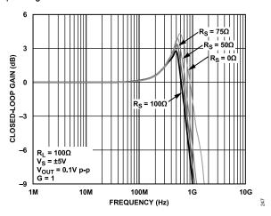
Figure 60. Small Signal Frequency Response for Various R<sub>S</sub> (SOIC)
