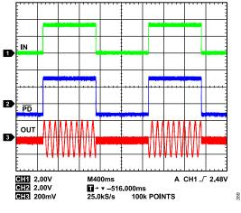
Figure 58. Power-Down Operation
