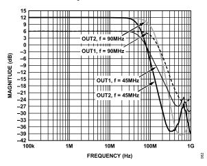
Figure 67. Low-Pass Filter Response
