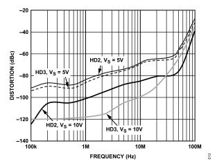
Figure 18. Distortion vs. Frequency for Various Supplies, V<sub>OUT</sub> = 2 V p-p
