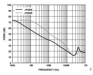
Figure 25. Power Supply Rejection Ratio (PSRR) vs. Frequency
