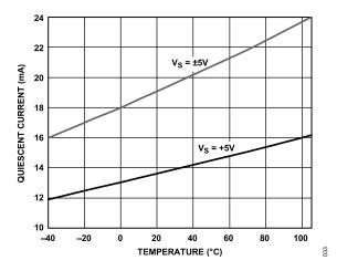
Figure 29. Quiescent Current vs. Temperature for Various Supply Voltages
