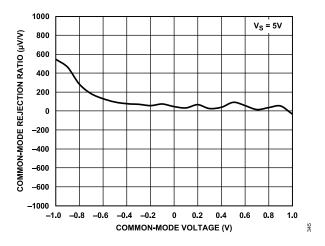
Figure 45. Common-Mode Rejection vs. Common-Mode Voltage, V<sub>S</sub> = 5 V
