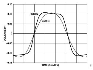
Figure 69. Small Signal Transient Response (Low-Pass Filter)
