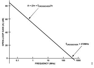
Figure 54. Open-Loop Gain vs. Frequency
