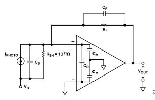
Figure 63. Wideband Photodiode Preamp
