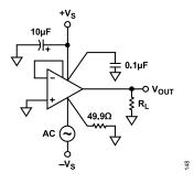
Figure 50. Negative Power Supply Rejection
