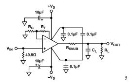
Figure 48. Capacitive Load Configuration
