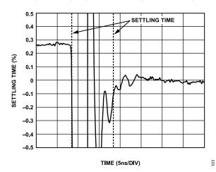
Figure 24. 0.1% Short-Term Settling Time
