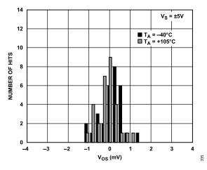
Figure 33. Input Offset Voltage Histogram over Temperature (V<sub>S</sub> =  $\pm$ 5 V), LFCSP Only
