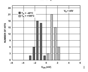
Figure 34. Input Offset Voltage Histogram over Temperature (V<sub>S</sub> =  $\pm$ 5 V), SOIC Only
