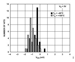
Figure 36. Input Offset Voltage Histogram over Temperature (V<sub>S</sub> = 5 V), LFCSP Only
