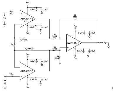
Figure 66. High Speed Instrumentation Amplifier
