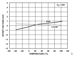
Figure 38. Offset Voltage vs. Temperature (V<sub>S</sub> = ±5 V)
