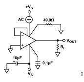
Figure 47. Positive Power Supply Rejection
