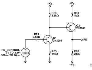
Figure 57. Power-Down Circuit
