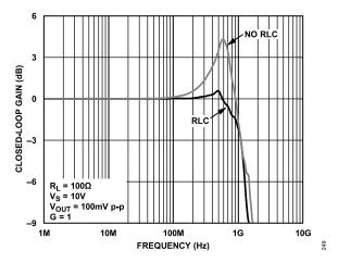
Figure 62. Frequency Response with RLC Circuit
