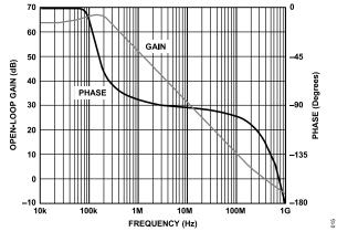
Figure 31. Open-Loop Gain and Phase vs. Frequency
