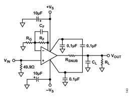
Figure 56. R<sub>SNUB</sub> or C<sub>F</sub> Used to Reduce Peaking
