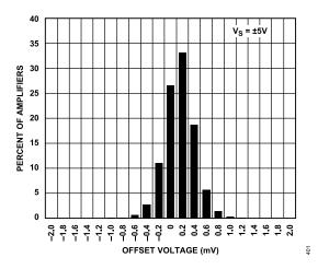
Figure 35. Input Offset Voltage Histogram (V<sub>S</sub> = ±5 V), SOIC Only
