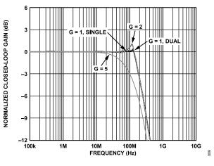
Figure 11. Large Signal Frequency Response for Various Gains
