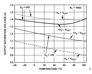
Figure 30. Output Saturation Voltage vs. Temperature
