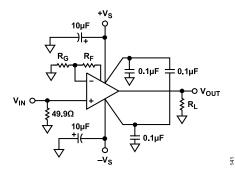
Figure 49. Noninverting Gain Configuration
