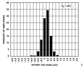
Figure 32. Input Offset Voltage Histogram (V<sub>S</sub> = ±5 V), LFCSP Only
