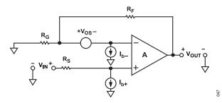
Figure 55. DC Errors of the Voltage Feedback Amplifier
