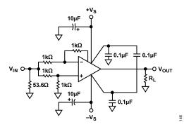
Figure 51. Common-Mode Rejection
