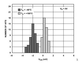
Figure 37. Input Offset Voltage Histogram over Temperature (V<sub>S</sub> = 5 V), SOIC Only
