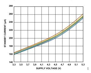
Figure 11. ADXL1001/ADXL1002 Standby Current vs. Supply Voltage
