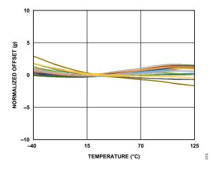
Figure 13. ADXL1002 Normalized Offset vs. Temperature
