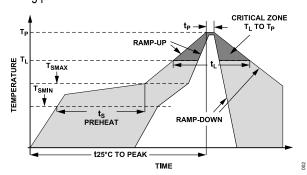
Figure 2. Recommended Soldering Profile
