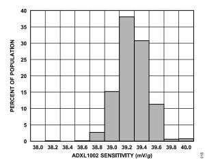
Figure 15. ADXL1002 Sensitivity Histogram at 25°C
