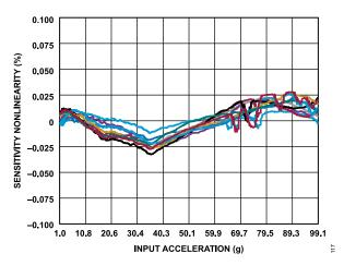
Figure 17. ADXL1001 Sensitivity Nonlinearity vs. Input Acceleration
