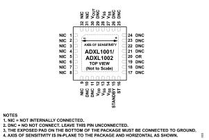
Figure 3. Pin Configuration
