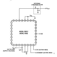
Figure 22. ADXL1001/ADXL1002 Application Circuit
