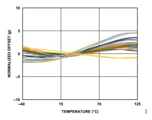
Figure 10. ADXL1001 Normalized Offset vs. temperature
