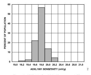
Figure 12. ADXL1001 Sensitivity Histogram at 25°C
