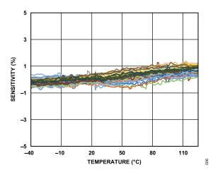
Figure 6. ADXL1001 Sensitivity vs. Temperature
