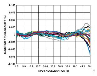
Figure 20. ADXL1002 Sensitivity Nonlinearity vs. Input Acceleration
