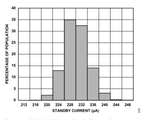
Figure 19. ADXL1001/ADXL1002 Standby Current Histogram at 5 V
