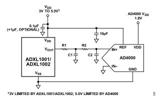
Figure 25. Application Circuit for the ADXL1001/ADXL1002
