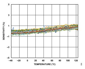
Figure 9. ADXL1002 Sensitivity vs. Temperature
