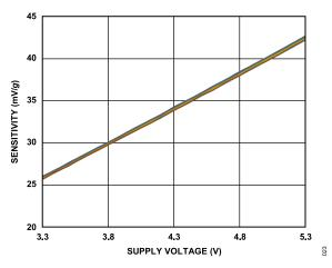
Figure 24. ADXL1002 Sensitivity vs. Supply Voltage
