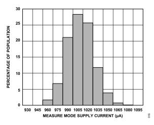
Figure 16. ADXL1001/ADXL1002 Measure Mode Supply Current Histogram at 5 V
