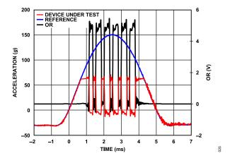
Figure 26. ADXL1001/ADXL1002 Behavior During a Continuous Overrange
