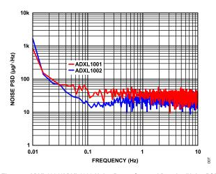
Figure 7. ADXL1001/ADXL1002 Noise Power Spectral Density (Noise PSD) Below 10 Hz
