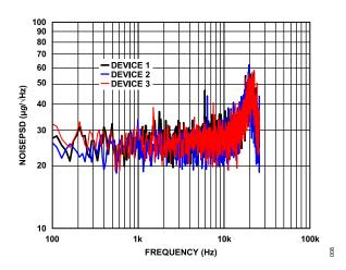
Figure 8. ADXL1002 Noise Power Spectral Density (PSD)
