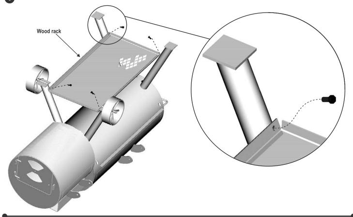
**MAKE SURE THAT LEG BOLTS ARE TIGHT ENOUGH SO THAT LEGS WON'T SLIP OFF OF POSTS.** With the assistance of a helper, roll the unit over the handle brackets and stand it up onto its legs. Once standing, fully tighten the four leg bolts.
