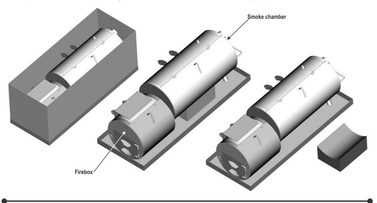
With one person on smoke chamber end, one person on firebox end, and one person holding both doors closed, roll the unti onto cardboard that was placed on the ground next to the unit. Unit should now be resting on its smoke chamber handle brackets with the leg posts pointing upward.
