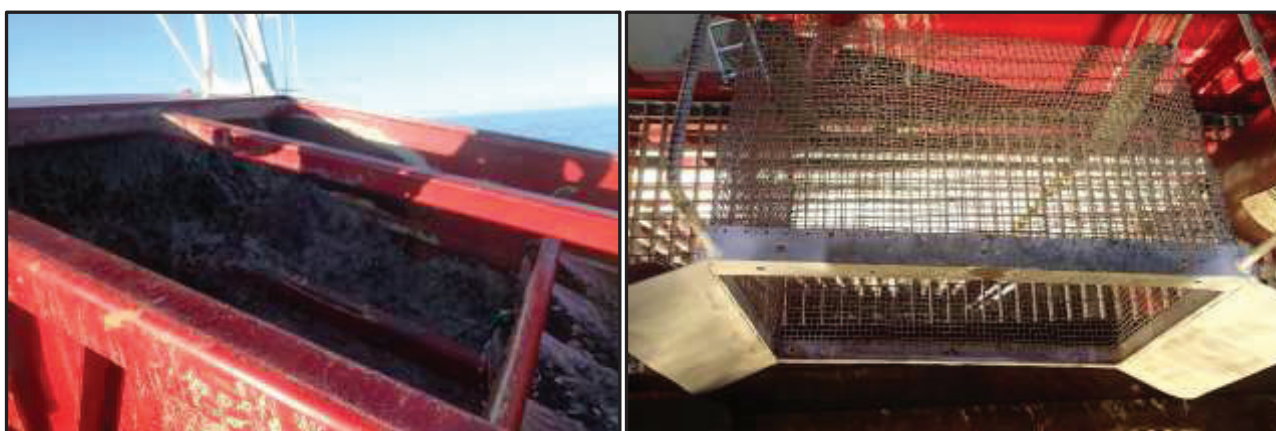
Figure 2.5 Sand and water pumped into the sieving system where sampling occurred (Left); and mesh basket used for sampling (right)
