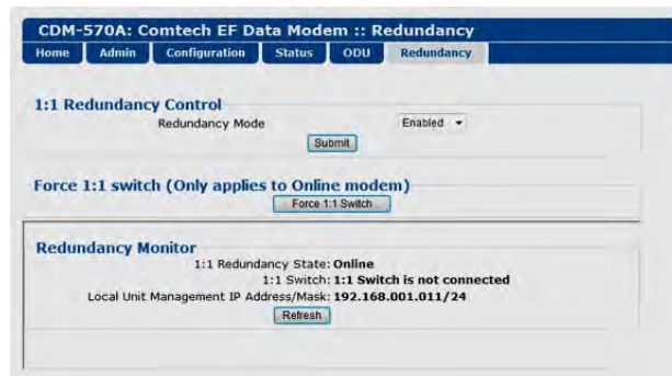
Ethernet HTTP (Web Server) Interface
