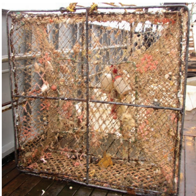
Figure 1.20 Steel pots are used to harvest many species of crabs in Alaska. Some pots, such as this one, measure 2 x 2 x 1 m and may weigh more than 300 kg. This pot was derelict for some time and has been heavily colonized by soft corals. Photo credit: Alaska Department of Fish and Game
