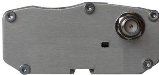
Figure 16 : Back side with option internal SIM chip S0532C
