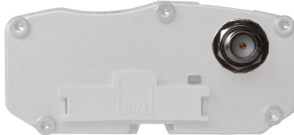
Figure 19 : External GSM antenna
