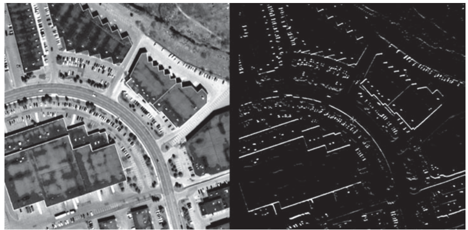
Figure 3. Example of automated edge enhancement. This algorithm removes the background image and records horizontal or near-horizontal lines as white. This is a high-resolution (1m pixels) image (source: author).
