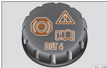
Fig. 215 Engine compartment: brake fluid reservoir cap.
