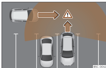
Fig. 172 Schematic representation of the rear cross traffic alert assistant: zone monitored around the vehicle while leaving a parking space.
