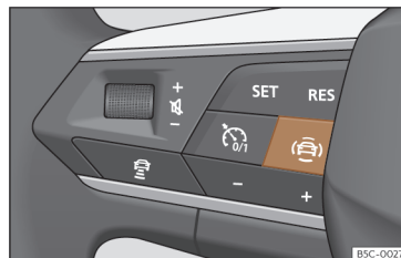
Fig. 62 Left side of the multifunction steering wheel: button for driver assistance systems (depending on versions).
