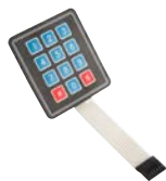
3 X 4 MATRIX MEMBRANE KEYPAD VMA300
