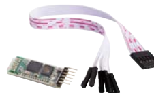
HC-05 TRANSMISSION MODULE VMA302
