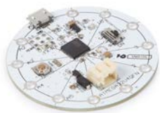
ATMEGA32U4 WEARABLE DEVELOPMENT BOARD VMA105
