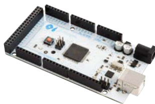
ATMEGA2560 MEGA DEVELOPMENT BOARD VMA101
