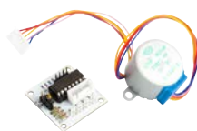
5 VDC STEPPER MOTOR WITH ULN2003 DRIVER BOARD VMA401
