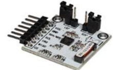
LIGHTNING SENSOR VMA343
