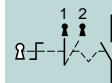
Selector switch 2-position stay put, key withdrawal from both positions N/O contact
