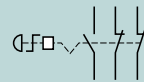
Mushroom head Emergency stop Turn to release, trigger action N/O + 2 N/C contacts
