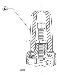
*Figure 11.* Optional Closing Cap (Only Available with the 1/4 in. / 6.4 mm Spring Case Vent)
