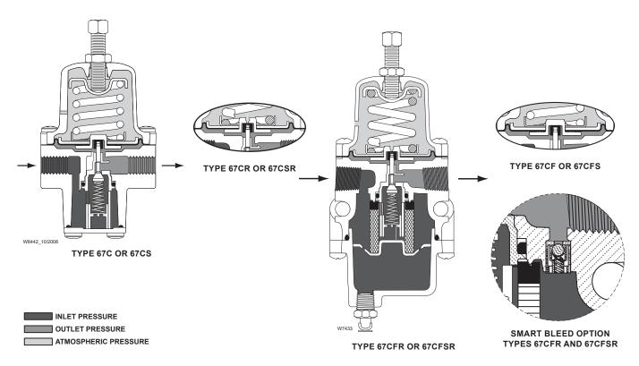
Figure 2. 67C Series Operational Schematics
