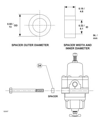
**Figure 13.** Spacer Diameter and Assembly (For Installing in an Existing Installation if the Mounting Bolts are Too Long)
