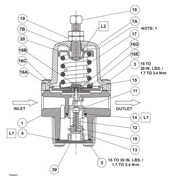
□ APPLY LUBRICANT (L) L1 = MULTI-PURPOSE POLYTETRAFLUOROETHYLENE (PTFE) LUBRICANT L2 = ANTI-SEIZE COMPOUND
