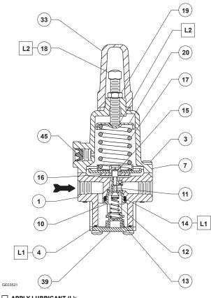
APPLY LUBRICANT (L): L1 = MULTI-PURPOSE POLYTETRAFLUOROETHYLENE (PTFE) LUBRICANT L2 = ANTI-SEIZE COMPOUND
