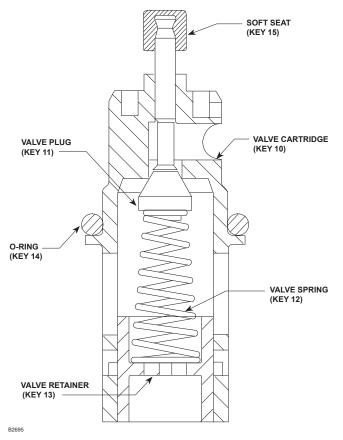
Figure 12. Valve Cartridge Assembly
