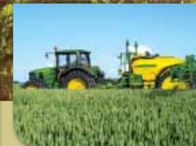
The compact design of the 700 Series trailed sprayers ensures a low centre of gravity for a high degree of stability in the field and on the road.
