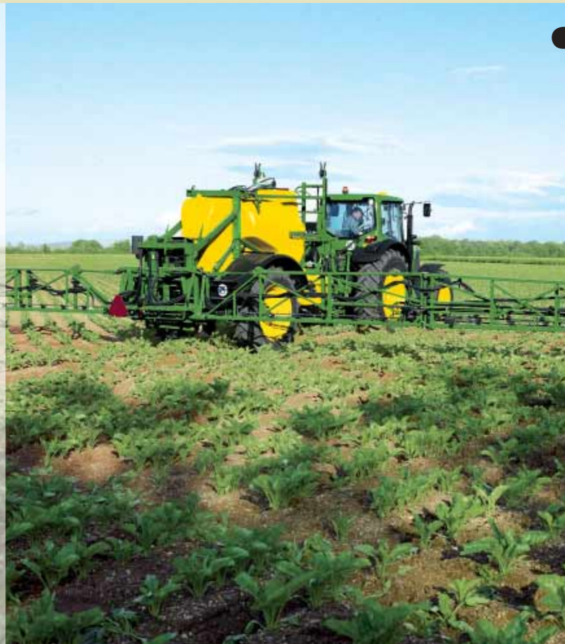
Hydraulic steering allows manual control of the drawbar, particularly useful when spraying on slopes to avoid down hill drift.
