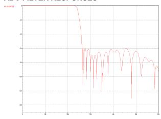
Figure 85 ADC Digital Filter Frequency Response (128OSR)
