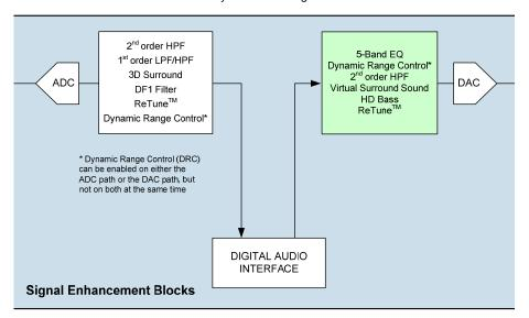
Figure 32 DAC Signal Enhancements
