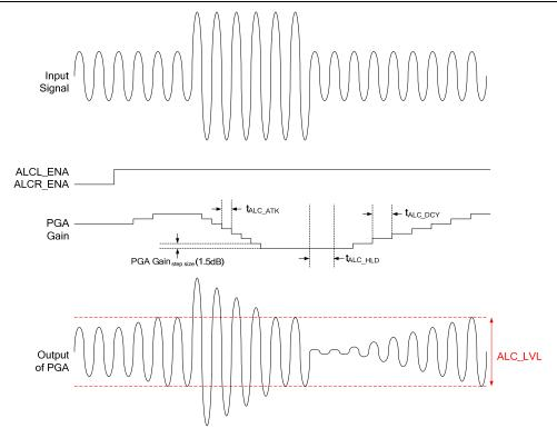
Figure 19 ALC Normal Mode Operation
