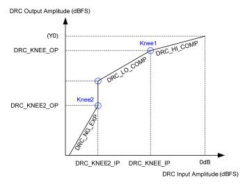
Figure 29 DRC Response Characteristic
