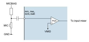
Figure 14 Microphone Input IN1 or IN4
