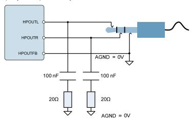
Figure 37 Zobel Network Components for HPOUTL and HPOUTR
