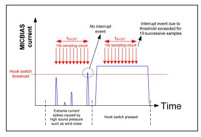
Figure 17 MICBIAS Hook Switch Detection Filtering
