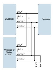
Figure 43 TDM with Processor as Master
