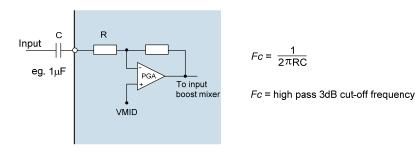
Figure 95 Audio Input Path DC Blocking Capacitor
