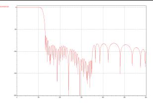
Figure 79 DAC Filter Response 22.05k Sample Rate
