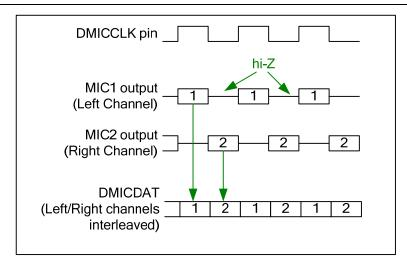
Figure 22 Digital Microphone Interface Timing
