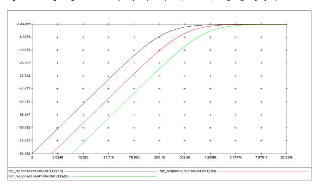
Figure 88 ADC Digital High Pass Filter Ripple (48kHz, Voice Mode, ADC\_HPF\_CUT=01, 10 and 11)
