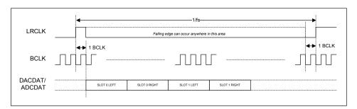
Figure 54 TDM in DSP Mode A
