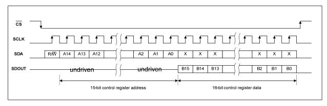
Figure 73 4-Wire Readback (Wired-'OR')
