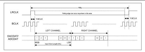
Figure 49 DSP Mode Audio Interface (mode A, LRCLK\_INV=0, Slave)
