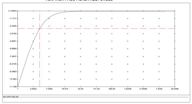
Figure 87 ADC Digital High Pass Filter Frequency Response (48kHz, Hi-Fi Mode, ADC\_HPF\_CUT[1:0]=00)
