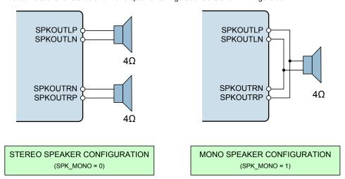
Figure 35 Mono and Stereo Speaker Output Configuration
