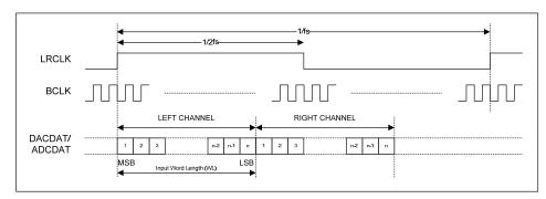
Figure 48 DSP Mode Audio Interface (mode B, LRCLK INV=1, Master)
