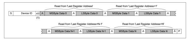
Figure 70 Multiple Register Read from Last Address using Auto-increment
