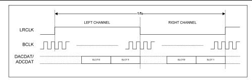
Figure 51 TDM in Right-Justified Mode
