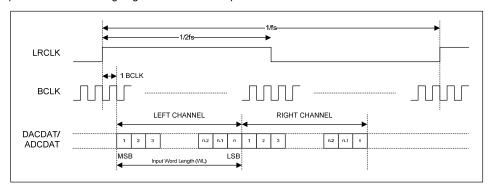
Figure 47 DSP Mode Audio Interface (mode A, LRCLK\_INV=0, Master)
