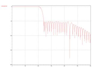
Figure 81 DAC Playback Filter Response for 32k Sample Rate
