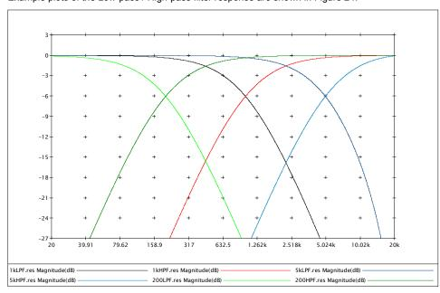
Figure 24 Low-pass / High-pass Filter Responses
