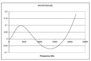
Figure 91 De-Emphasis Digital Filter Response (44.1kHz)
