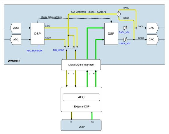
Figure 31 T-Loopback Signal Paths
