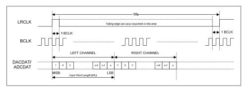
Figure 50 DSP Mode Audio Interface (mode B, LRCLK\_INV=1, Slave)
