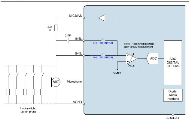
Figure 18 Multiple Hook Switch Detection
