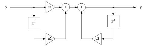
Figure 27 Direct-Form 1 Standard Filter Structure
