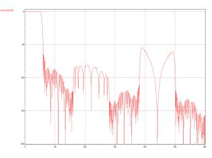
Figure 75 DAC Filter Response 8k Sampling Rate
