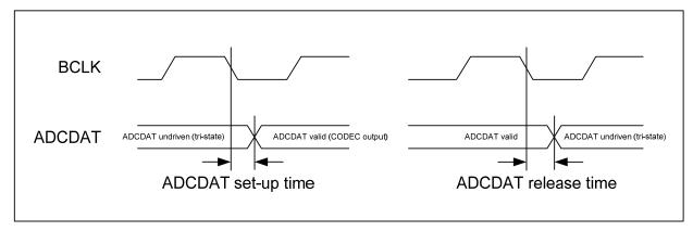
Figure 5 Audio Interface Timing - TDM Mode
