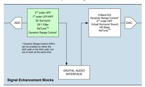
Figure 23 ADC Signal Path Enhancements
