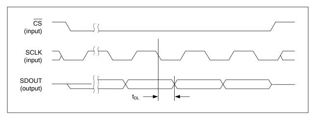
Figure 10 Control Interface Timing - 4-wire (SPI) Control Mode (Read Cycle)
