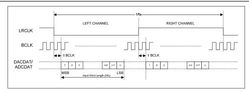
Figure 46 I2S Justified Audio Interface (assuming n-bit word length)
