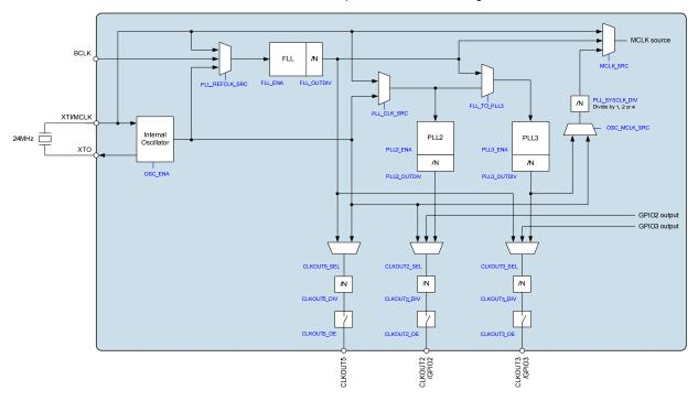
Figure 59 Clock Generation Block Diagram
