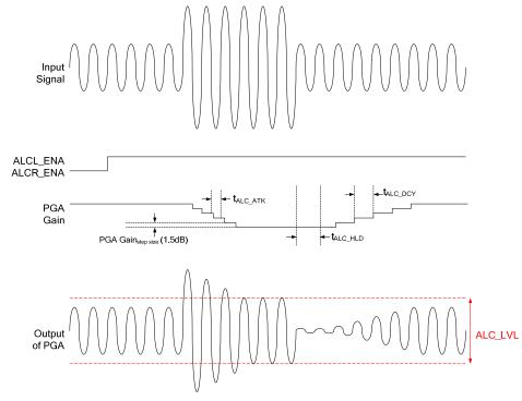
Figure 20 ALC Limiter Mode Operation
