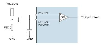
Figure 15 Microphone Input IN2 or IN3
