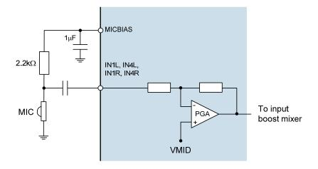
Figure 96 Single Ended Microphone Connection
