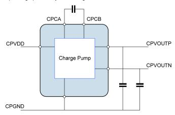
Figure 38 Charge Pump External Connections
