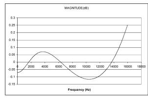
Figure 89 De-Emphasis Digital Filter Response (32kHz)
