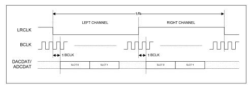
Figure 53 TDM in I<sup>2</sup>S Mode
