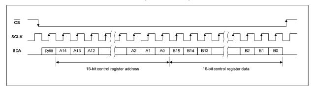
Figure 71 3-Wire Serial Control Interface
