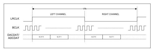
Figure 52 TDM in Left-Justified Mode
