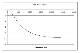
Figure 93 De-Emphasis Digital Filter Response (48kHz)
