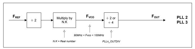
Figure 62 PLL Frequency Control
