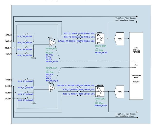
Figure 13 Analogue Input Signal Path
