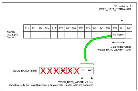
Figure 74 Control Write Sequencer Example
