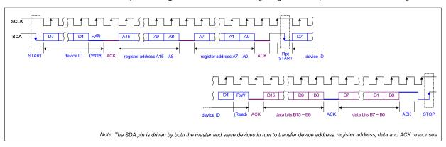
Figure 65 Control Interface 2-wire (I2C) Register Read
