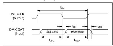
Figure 2 Digital Microphone Interface Timing
