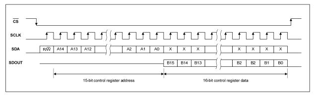
Figure 72 4-Wire Readback (CMOS)
