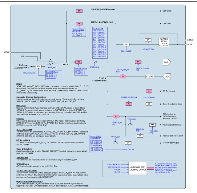
Figure 58 SYSCLK and Internal Clocking Scheme
