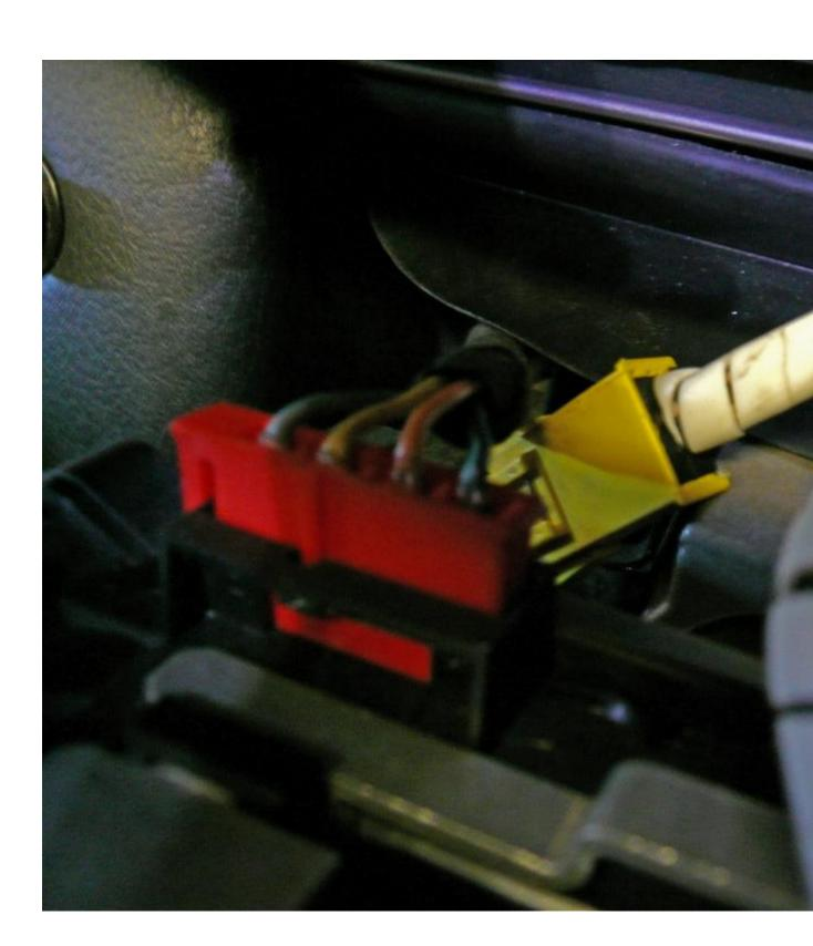
The exposed indicator console can now be removed by firstly unplugging the 5 electrical connectors that go to it
