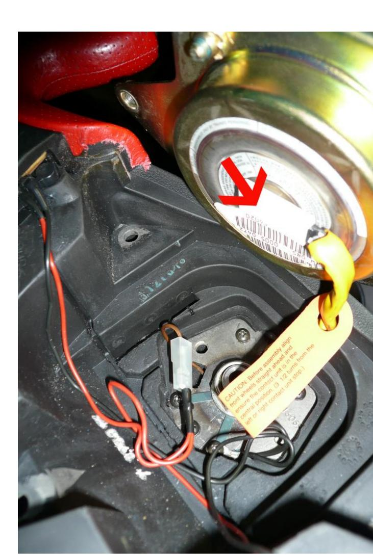
Carefully unplug the cable off the airbag. Put aside the disconnected airbag face-up at a safe place.
