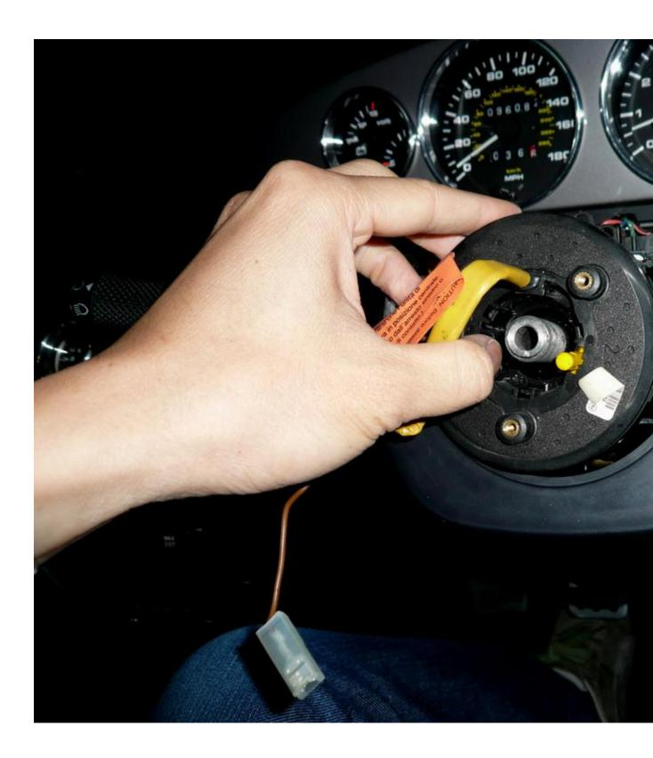
You can either push the clock-spring aside and leave it connected or remove it completely by unplugging the yellow socket that is found at the top of the indicator console shown here.
